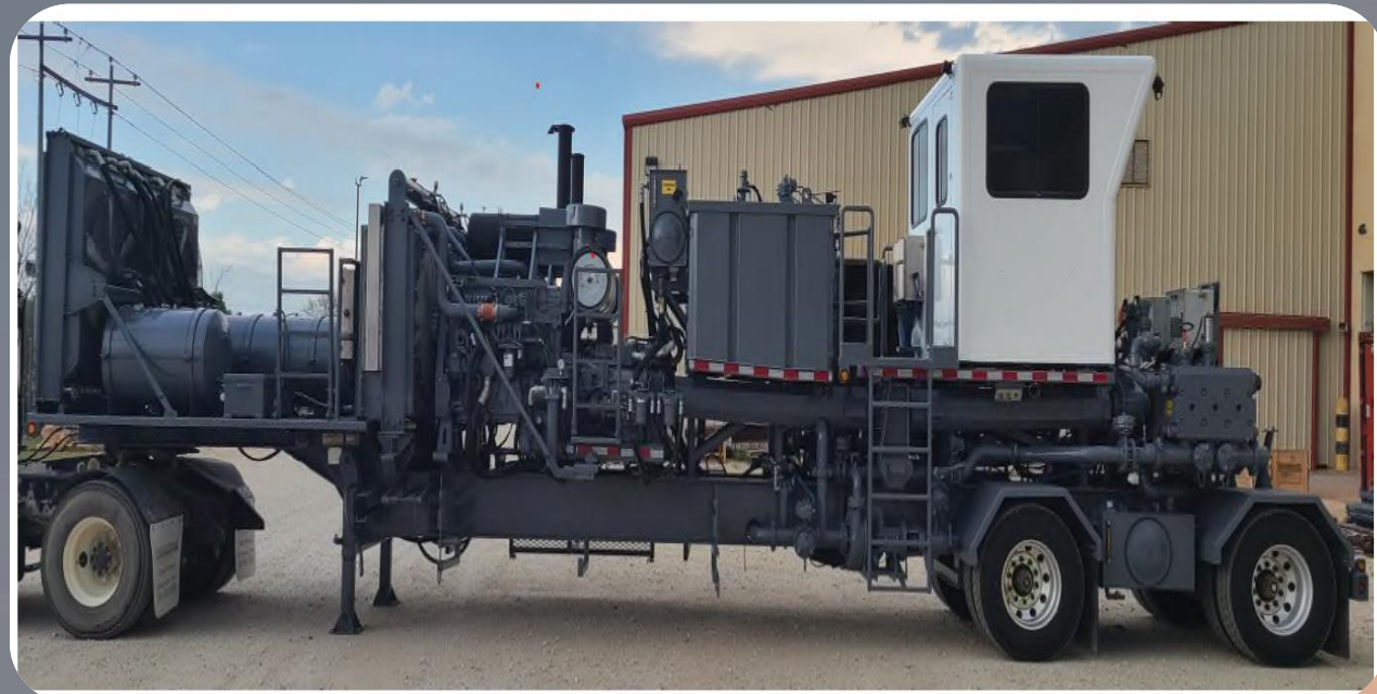
Twin Pump 1100 HHP Trailer Mounted Unit
