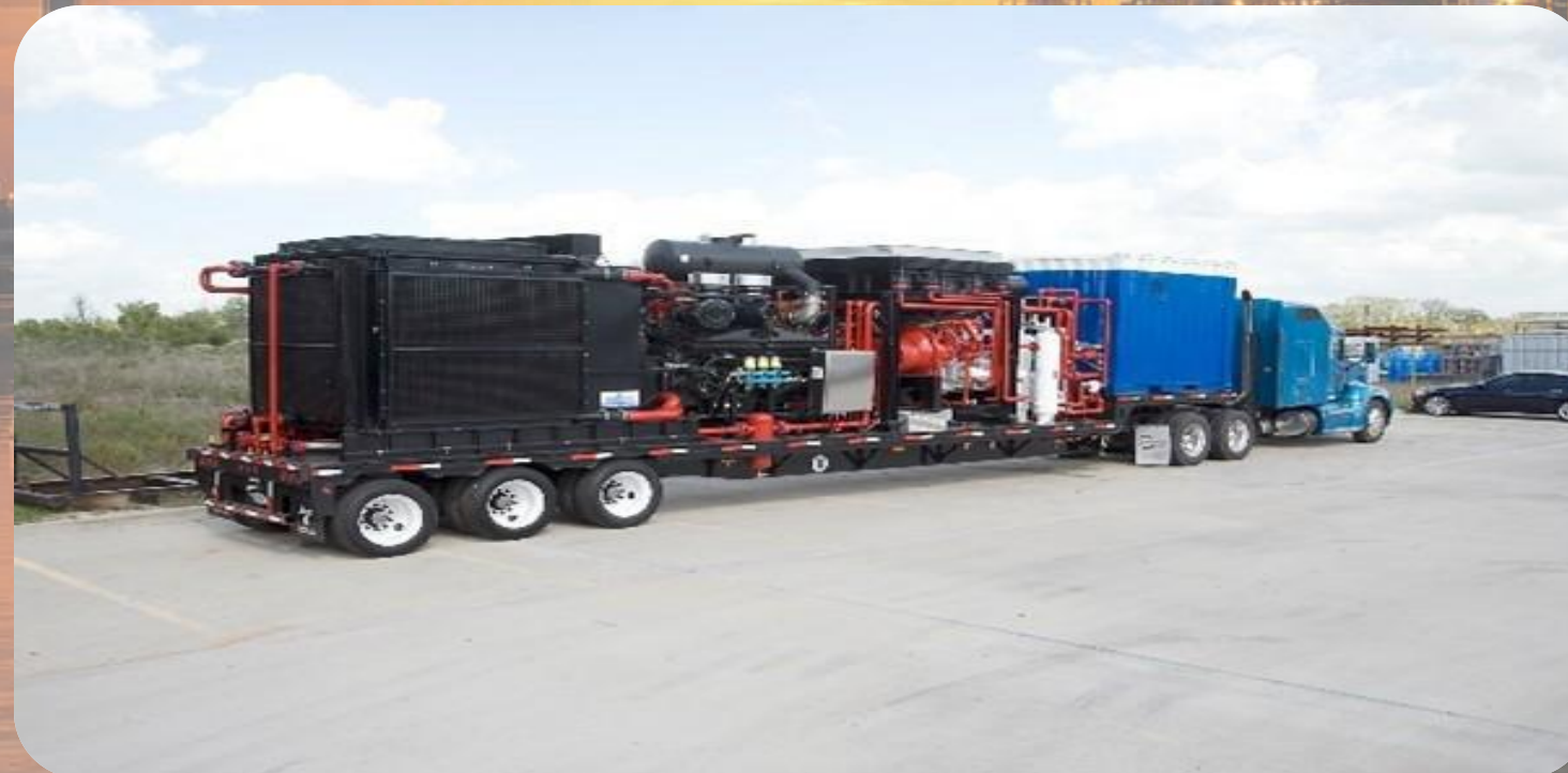
NGU-Nitrogen Generation Unit
